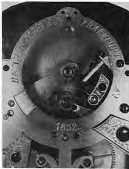
Figure 4. Close-up view of Meek's Escapement. Courtesy of Orville R. Hagans.
