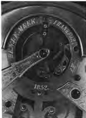
Figure 3. Close-up view of Meek's Compensation Balance and Escapement. Courtesy of Orville R. Hagans.
