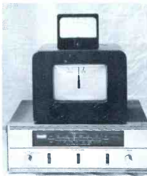
The original Hamlin single channel field strength meter, made by modifying a pilot FM tuner, is shown atop the latest piece of Hamlin-designed equipment, an all transistorized FM multiplex stereo tuner.
