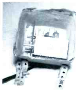
This CATV "museum piece" is the first antenna preamp, mixer, IF amplifier from the original South Bend system. It was bracketed to an apple box which was fastened to the mast. Underground RG59 connected it to first IF "reamplifier" in basement of house about forty feet away.
