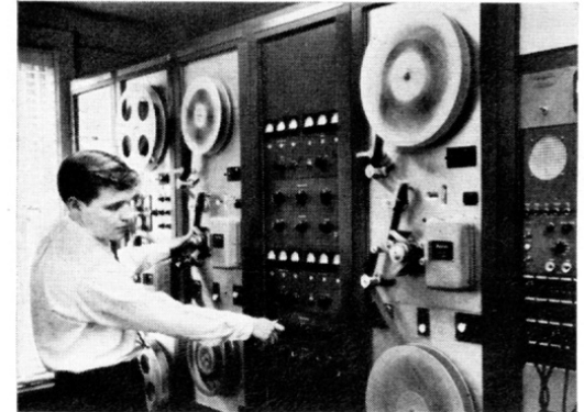
Performers are recorded on dual 35mm magnetic film recorders (above). Magnetic film, although superior to conventional magnetic recording tape in most respects, is not used universally in the recording industry because of its high cost: roughly 15 times the price of magnetic tape.
