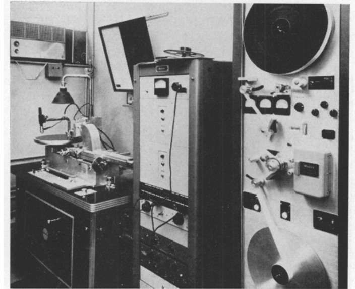
FIG. 7. One of the Everest's disk recording rooms showing a special Westrex 35-mm three-track reproducer and associated equipment.
